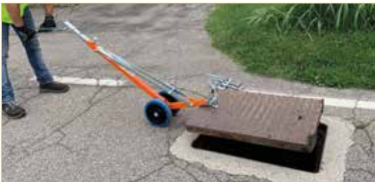
Use 3: mechanical opening with locking clamps.
