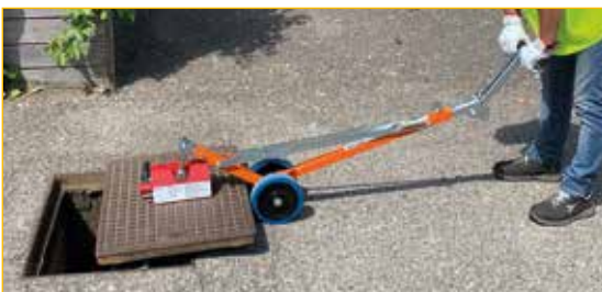
Use 4: magnetic opening with magnet permanent (PM400 or PM500) for very heavy manhole cover.
