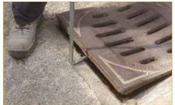
The "D" shaped handle provides a fulcrum point to facilitate the lifting operation.
