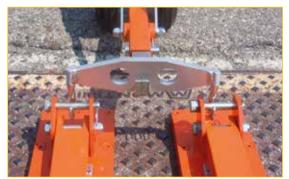
Shown in picture the wheeled lever engaged with two **CL10** connected by the "bridge".
