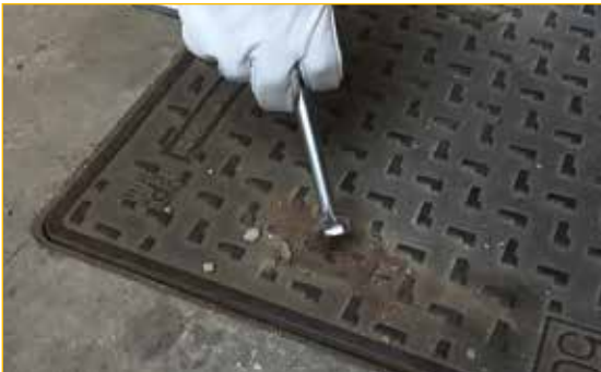
Configuration 3: "T" shaped end to be used as a flap or insertion key in the slots.
