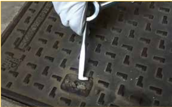
Configuration 2: L - shaped end for scraping in the inside of the slot and release the rotation for opening the lid.
