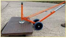
Lifting with wheeled levers APS80 or APS90
