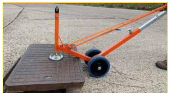
Lifting with wheeled levers APS80 or APS90
